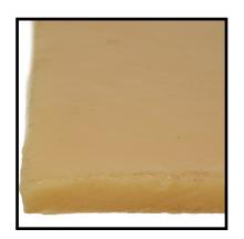
SynTissue bulk fat is very soft and lubricious. This fat is also much more friable than the subcutaneous grade due to a lower fiber content. Standard product is a  $20 \text{cm} \times 20 \text{cm}$  plate with a nominal thickness of 5.0 mm.
